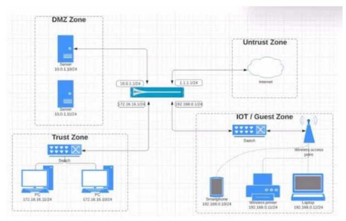
View the diagram. What is the most restrictive, yet fully functional rule, to allow general Internet and SSH traffic into both the DMZ and Untrust/Internet zones from each of the IOT/Guest and Trust Zones? A)
