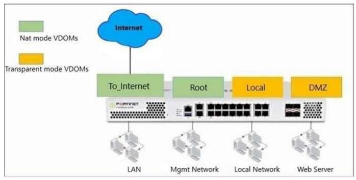
The Root and ToInternet VDOMs are configured in NAT mode. The DMZ and Local VDOMs are configured in transparent mode. The Root VDOM is the management VDOM. The ToInternet VDOM allows LAN users to access the internet. The ToInternet VDOM is the only VDOM with internet access and is directly connected to ISP modem. With this configuration, which statement is true?
