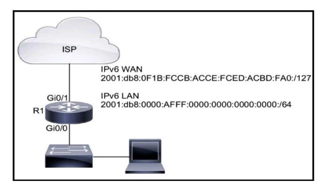
IPv6 must be implemented on R1 to the ISP The uplink between R1 and the ISP must be configured with a manual assignment, and the LAN interface must be self-provisioned Both connections must use the applicable IPv6 networks Which two configurations must be applied to R1? (Choose two.)
