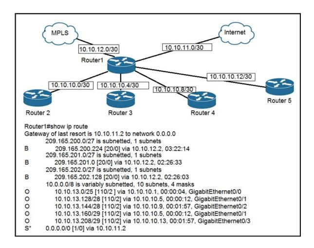
Refer to the exhibit. To which device does Router1 send packets that are destined to host 10.10.13.165?
