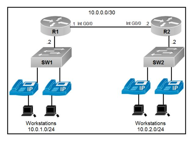
An engineer is asked to configure router R1 so that it forms an OSPF single-area neighbor relationship with R2. Which command sequence must be implemented to configure the router?
