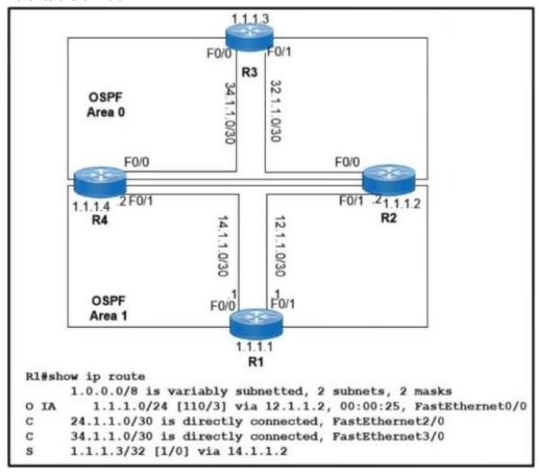
Which two values does router R1 use to determine the best path to reach destinations in network 1,0.0.0/8? (Choose two.)
