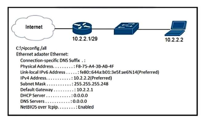
A newly configured PC fails to connect to the internet using TCP port 80 to www cisco com Which setting must be modified for the connection to work?
